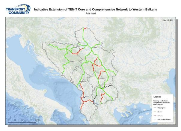
Figure 8. Map of axle load in tons/axle on Core and Comprehensive Network
