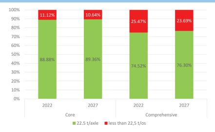
Figure 38. Western Balkans Rail network axle load progress forecast for 2027
