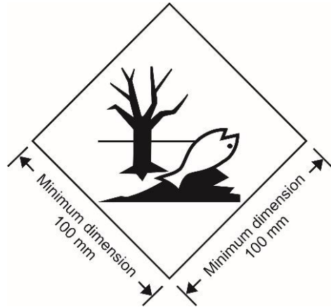
Environmentally hazardous mark
